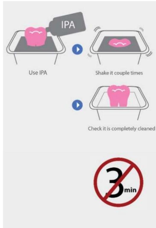
**2. Cleaning with IPA** You can use IPA instead of warm tap-water to clean excess resins, but more than 3 minutes exposure to IPA will result in cracks in prints. Just put prints into IPA and shake it couple times and remove it from IPA. This will speed up washing and drying processes.
